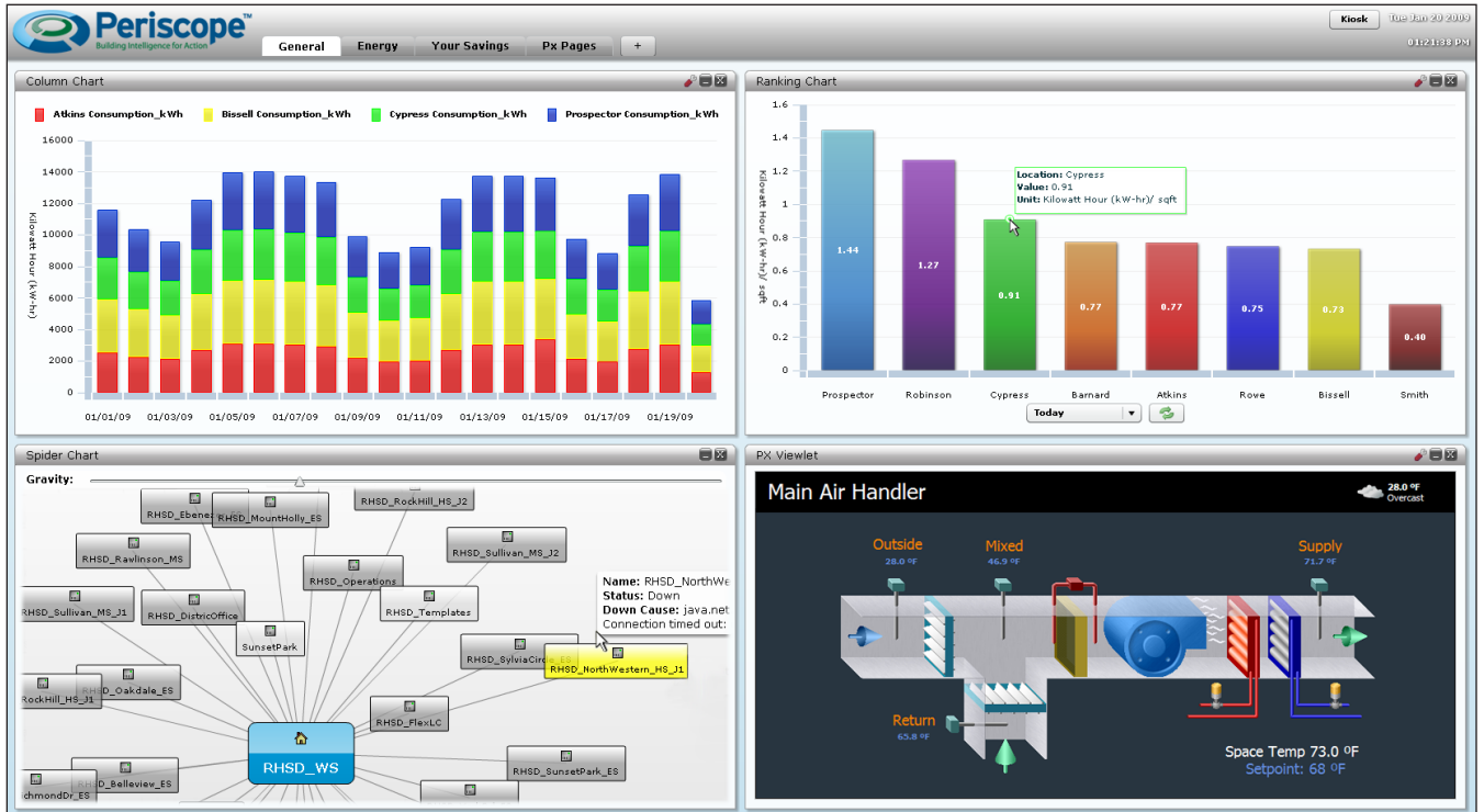
The Dashboard - Periscope’s interface can easily be modified with a library of “viewlets” to suit the preferences of any user. The viewlets can then be configured in a variety of ways, allowing each user to create a custom-tailored display.
